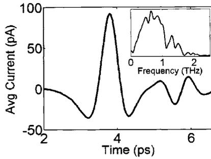
FIG. 2. THz pulse from sample arm (A). The inset shows the spectral amplitude,  $S(\omega)$  obtained by a numerical Fourier transform. The reference arm spectrum,  $R(\omega)$ , is nearly identical. The oscillations after the pulse and valleys in the spectrum are due to atmospheric water vapor.
