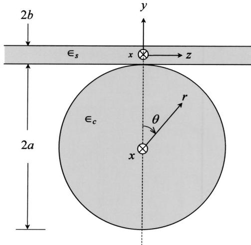
Fig. 7. Coordinate system of the slab-cylinder coupling structure.
