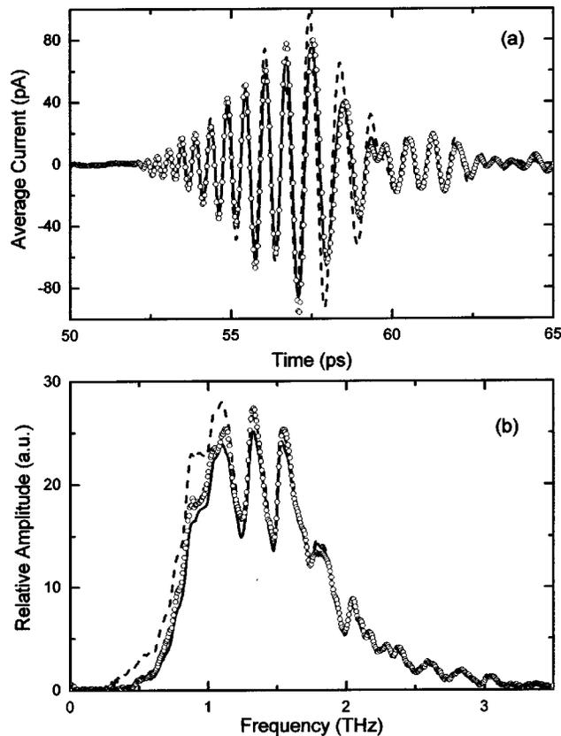
Fig. 4. (a) Main transmitted pulses of Fig. 3 and, (b) their corresponding spectra. The dashed curves represent the reference scan, the open circles represent the sample scan, and the solid curves are the calculation results for the sample scan.
