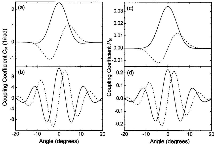
Fig. 8. Coupling coefficients for the slab  $\text{TM}_0$  mode and  $\text{WG}_1$  mode at 1.0 and 0.5 THz. The solid curves are real parts and the dashed curves represent imaginary parts. (a)  $C_{01}$  at 1 THz. (b)  $C_{01}$  at 0.5 THz. (c)  $P_{01}$  at 1 THz. (d)  $P_{01}$  at 0.5 THz.
