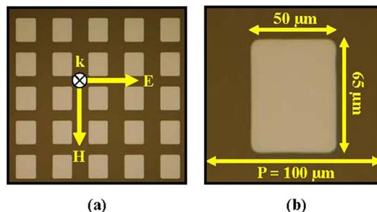
Fig. 1. (Color online) Optical images of (a) a periodic subwavelength YBCO hole array on a sapphire substrate and (b) a unit cell with geometric dimensions.
