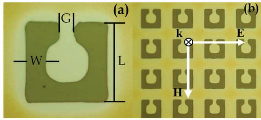
FIG. 1. (Color online) Microscopic image of (a) YBCO MM unit cell with structural parameters,  $W=8\ \mu\text{m}$ ,  $G=5\ \mu\text{m}$ , and  $L=32\ \mu\text{m}$  and (b) MM array with a periodicity of  $P=52\ \mu\text{m}$ . The incident E field is polarized parallel to the gap of the single SRRs.
