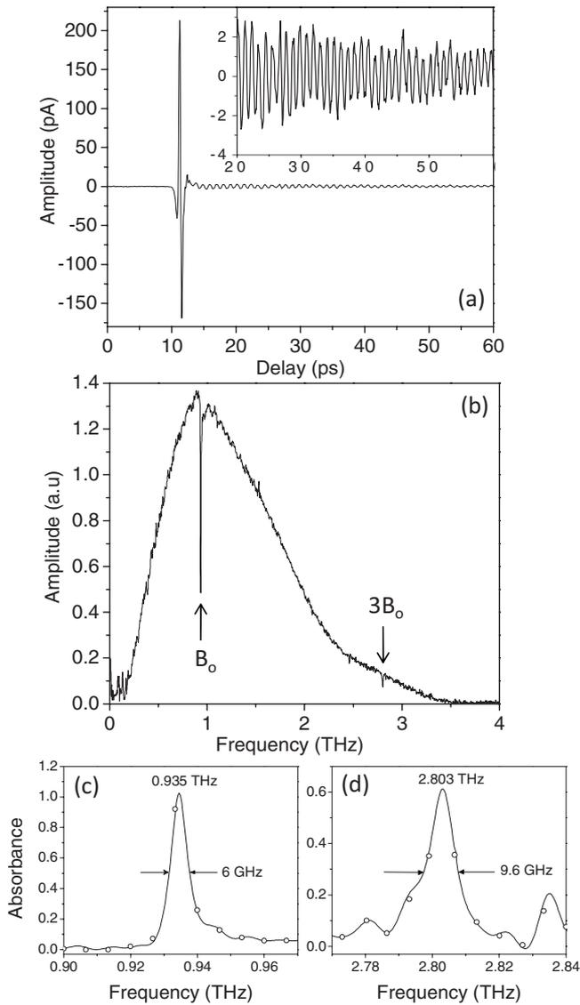
FIG. 2. (a) Output terahertz pulse from type A Bragg waveguide. (b) Transmission spectrum of output pulse. [(c) and (d)] Waveguide absorbance spectrum zoomed in at the fundamental Bragg frequency  $B_0$  and its third harmonic  $3B_0$ . Open circles indicate nonzero-padded data points separated by 6.7 GHz.
