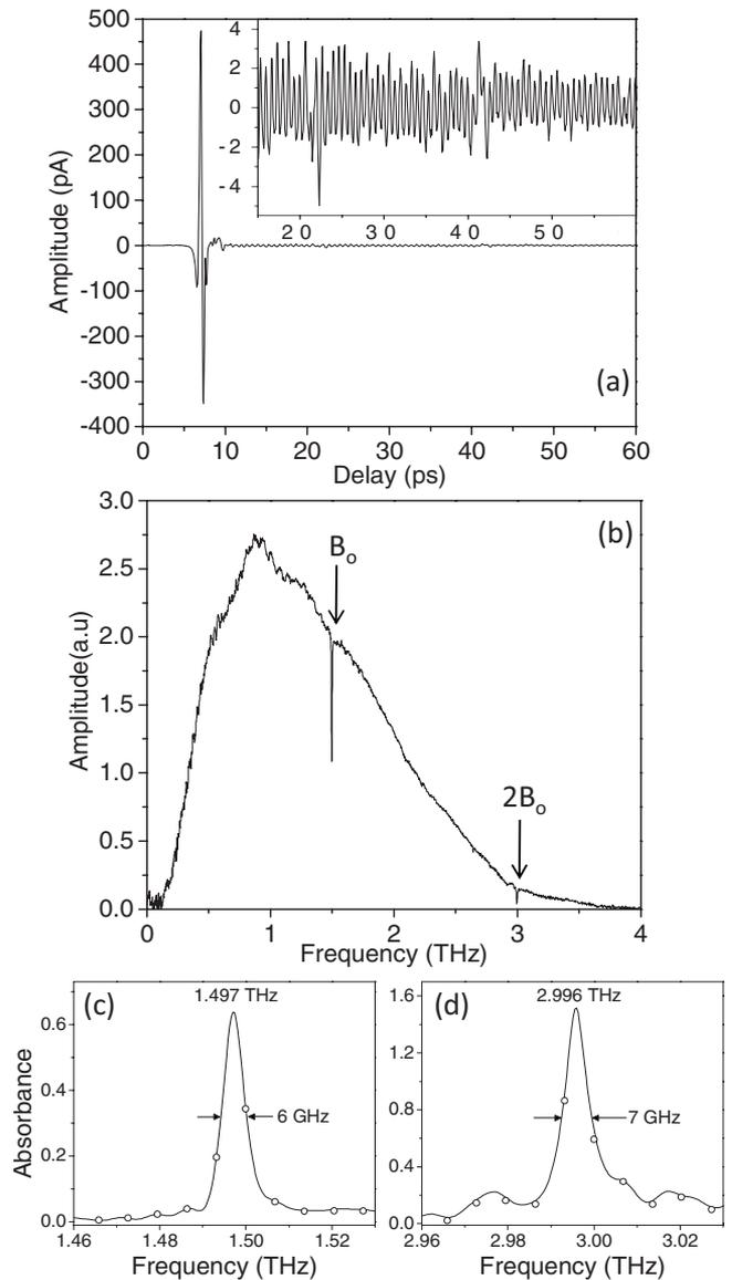
FIG. 3. (a) Output terahertz pulse from type B Bragg waveguide. (b) Transmission spectrum of output pulse. [(c) and (d)] Waveguide absorbance spectrum zoomed in at the fundamental Bragg frequency  $B_0$  and its second harmonic  $2B_0$ . Open circles indicate nonzero-padded data points separated by 6.7 GHz.
