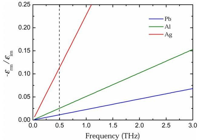
Fig. 3. (Color online) Frequency-dependent Drude ratio,  $-\epsilon_{rm}/\epsilon_{im}$  of Pb, Al, and Ag in the terahertz regime [11,12]; the vertical dashed line indicates the LC resonance frequency 0.5 THz.
