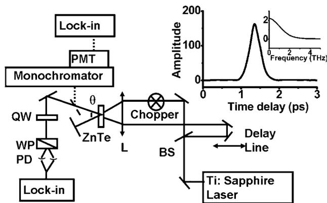
FIG. 1. Right: femtosecond Kerr-lens autocorrelation: time-domain trace and corresponding amplitude spectra, Left: the pump-probe experimental setup.
