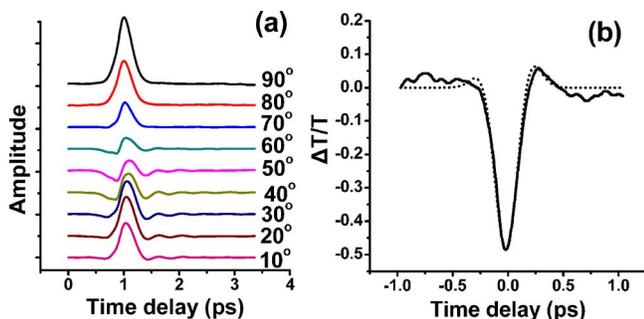
FIG. 2. (Color online) (a) The recorded signal using balanced detection part from  $10^\circ\sim 90^\circ$ , (b) the recorded signal (solid line) using spectrally resolved two-beam coupling at  $90^\circ$ , and the dotted line is theoretical fit data by setting the nonlinear refractive coefficient  $n_2=7\times 10^{-18}\text{ m}^2/\text{W}$  and the nonlinear absorption coefficient  $\beta=38\text{ cm/GW}$ .
