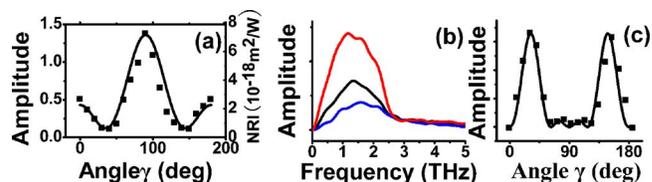
FIG. 4. (Color online) (a) Femtosecond Kerr-lens autocorrelation signal at zero frequency by rotating the ZnTe crystal every  $10^\circ$  along the (110) direction and nonlinear refractive index coefficient at every degree. (b) The pure terahertz spectra minus Kerr-lens autocorrelation amplitude spectra. (c) Terahertz signal intensity as a function of angle.
