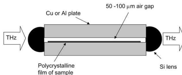
FIGURE 2 Parallel-plate waveguide.
