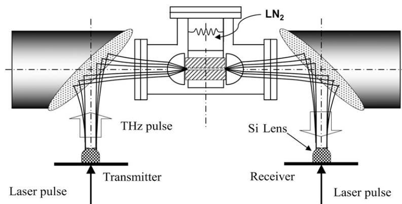
FIGURE 3 Waveguide THz-TDS.
