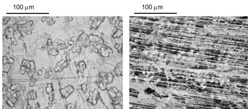
FIGURE 10 Optical micrographs of L-alanine polycrystalline films. (Left) Film resulting from drop-cast of water solution onto Cu plate. (Right) Corresponding drop-cast on Al plate. Micrograph on right is negative for clarity.
