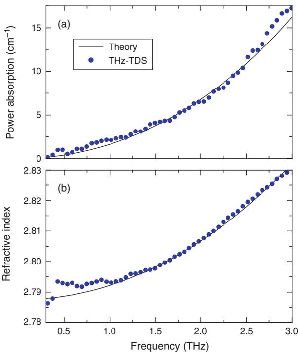
**Fig. 3.** (a) Comparison of measured power absorption  $\alpha$  with that obtained from pseudo-harmonic theoretical fitting for single-crystal ZnO; (b) measured refractive index and the theoretical fitting.
