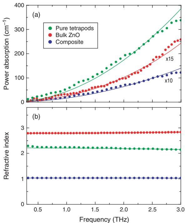
**Fig. 9.** Comparison of (a) measured power absorption, and (b) refractive index of pure ZnO tetrapods with that of bulk single-crystal ZnO and the tetrapod-air composite. The solid curves are corresponding theoretical fit to the data.
