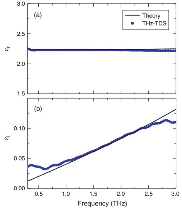
**Fig. 11.** Complex dielectric constant of ZnS nanoparticles: (a) measured real part of dielectric constant  $\epsilon_r$  and the theoretical fitting; (b) measured imaginary dielectric constant  $\epsilon_i$  and the theoretical fitting.
