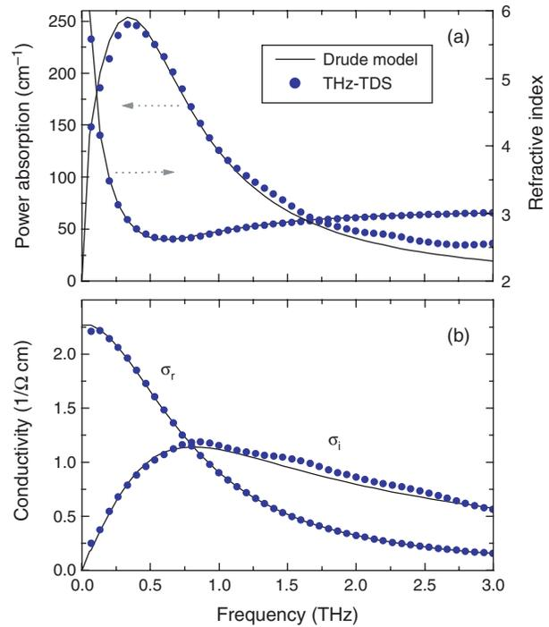
**Fig. 2.** Comparison of measured results of GaN with Drude model fitting. (a) Power absorption coefficient  $\alpha$  and the real part of refractive index  $n_r$ ; (b) complex electric conductivity  $\sigma_r$  and  $\sigma_i$ .
