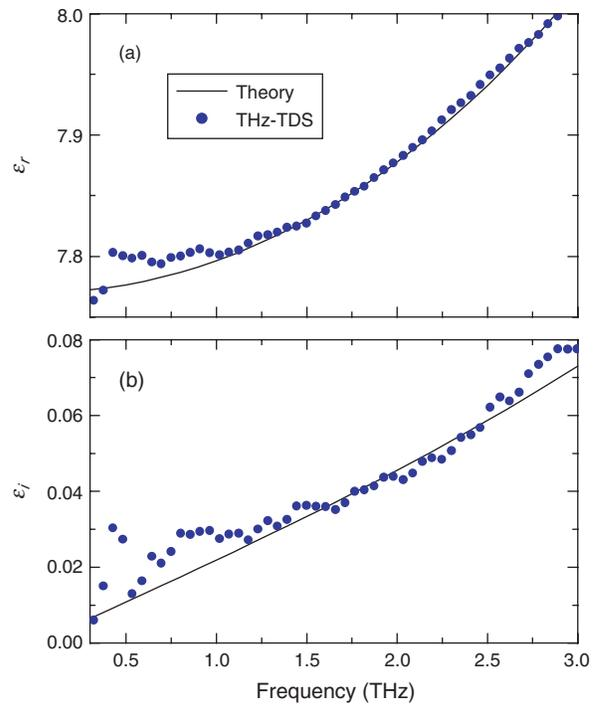
**Fig. 4.** Complex dielectric constant of single-crystal ZnO: (a) measured real part of dielectric constant  $\varepsilon_r$  and the theoretical fitting; (b) measured imaginary dielectric constant  $\varepsilon_i$  and the theoretical fitting.
