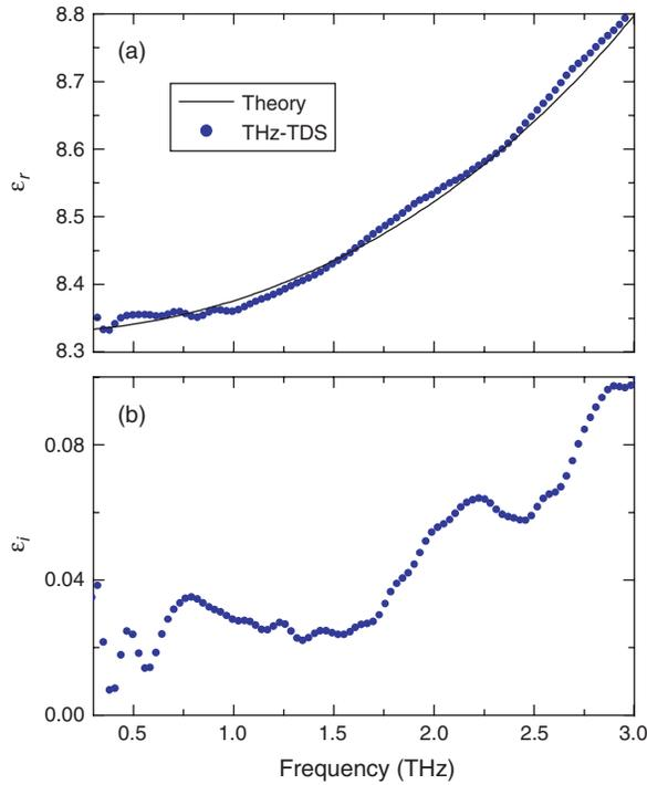
**Fig. 6.** Complex dielectric constant of single-crystal ZnS: (a) measured real part of dielectric constant  $\epsilon_r$  and the theoretical fitting; (b) measured imaginary dielectric constant  $\epsilon_i$ .
