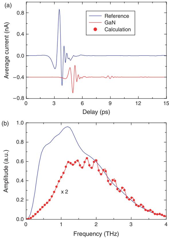
**Fig. 1.** (a) THz-TDS measured reference pulse and sample pulse with reflections (vertically displaced by  $-0.4$  nA) for free-standing GaN; (b) Fourier-transformed amplitude spectra of the reference and sample (multiplied by  $2\times$ ) pulses. The dots represent the calculated sample spectrum from the reference.
