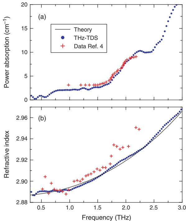
**Fig. 5.** (a) Comparison of measured results for the absorption of single-crystal ZnS with: the data from Ref. [4]; (b) comparison of measured refractive index of single crystal ZnS with: the values calculated using the damped harmonic oscillator model and the data from Ref. [4].
