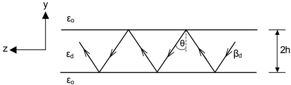
Figure 6-1. Ray path due to total internal reflection.
