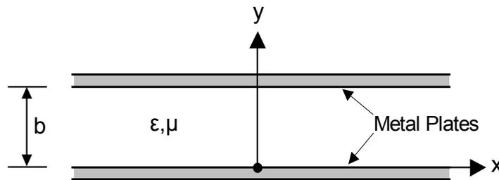
Figure 4-4. Transverse cross-section of the parallel-plate waveguide.
