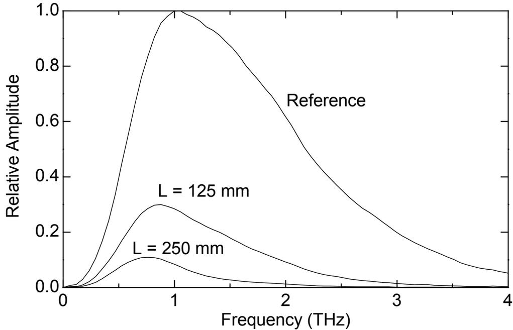
Figure 5-3. Amplitude spectra of the isolated pulses.
