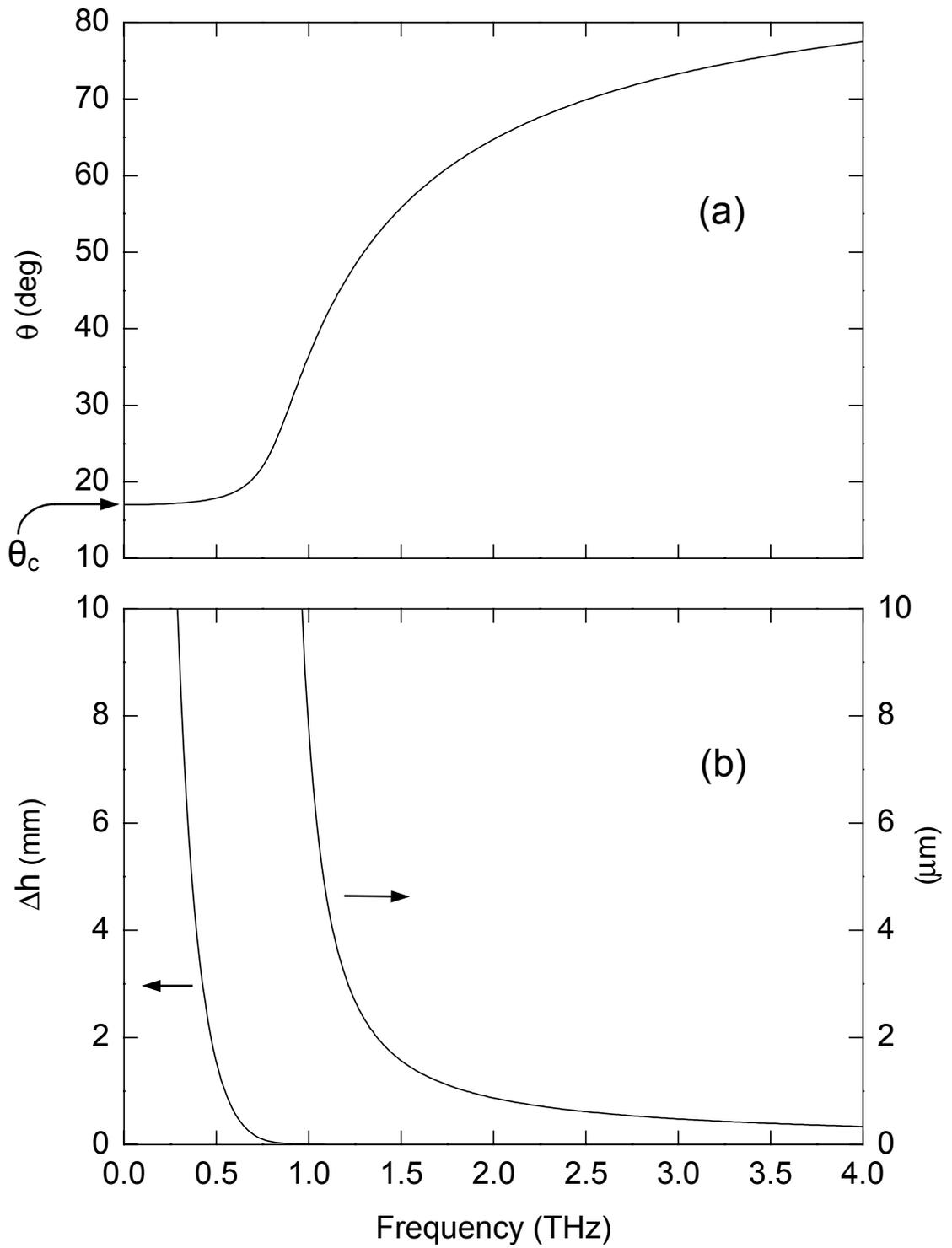
Figure 6-4. (a) Variation of  $\theta$  with frequency for the  $\text{TM}_0$  mode. (b) Variation of  $\Delta h$  with frequency, plotted to two different vertical scales. The curve on the left corresponds to mm, and the curve on the right corresponds to  $\mu\text{m}$ .
