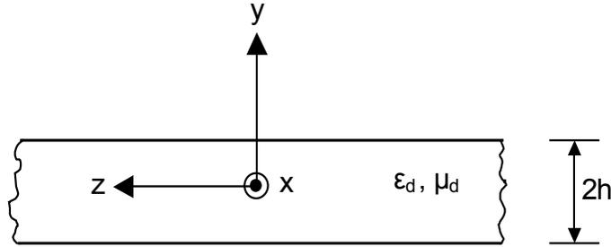
Figure 3-5. Longitudinal cross-section of the dielectric slab waveguide.
