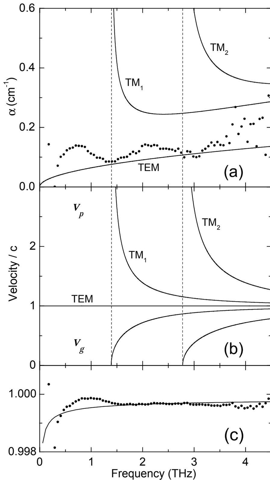
Figure 4-6. Amplitude absorption constant (a), and phase and group velocity (b), for the first three modes. Cutoff conditions are shown by the dashed lines. (c) Blown-up view of (b) in the vicinity of unity. Experimental values are shown by the dots.
