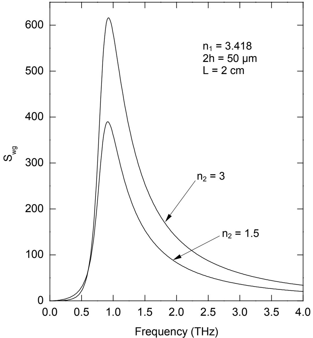
Figure 6-7. Variation of the waveguide sensitivity  $S_{wg}$  with frequency, for two different film indices. Upper curve corresponds to an index  $n_2 = 3$ , and the lower curve corresponds to  $n_2 = 1.5$ . The lower curve is identical to the one derived using the ray optics approach.
