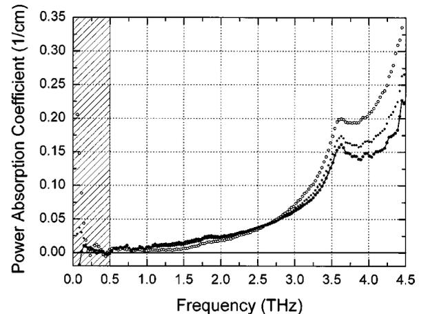
Fig. 5. Measured power absorption coefficients  $\alpha_{21}(\omega)$  open circles,  $\alpha_{31}(\omega)$  dots, and  $\alpha_{32}(\omega)$  connected dots. These measurements are considered accurate between 0.5 THz and 4.5 THz.
