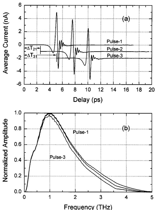
Fig. 3. (a) Measured transmitted pulses: Pulse 1, (Pulse 2)/( $t_{12}t_{21}$ ), (Pulse 3)/( $t_{12}r_{21}r_{21}t_{21}$ ). (b) Amplitude spectra for Pulse 1, (Pulse 2)/( $t_{12}t_{21}$ ), (Pulse 3)/( $t_{12}r_{21}r_{21}t_{21}$ ).
