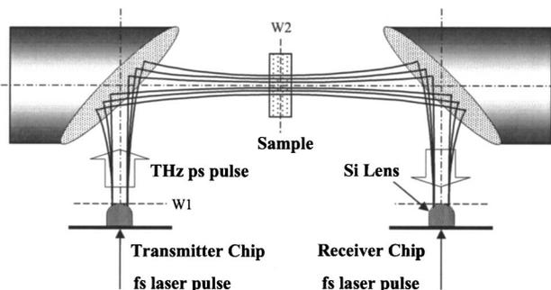
Fig. 1. The optoelectronic THz-TDS confocal quasi-optic system.
