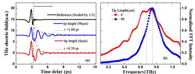
Fig. 4. (Color online) (a) Time-domain terahertz pulses through free space and the bow-tie arrays with tip lengths of 0 and  $90 \mu\text{m}$ , and (b) Fourier-transformed normalized spectra of the time-domain waveforms after 3.3 ps.
