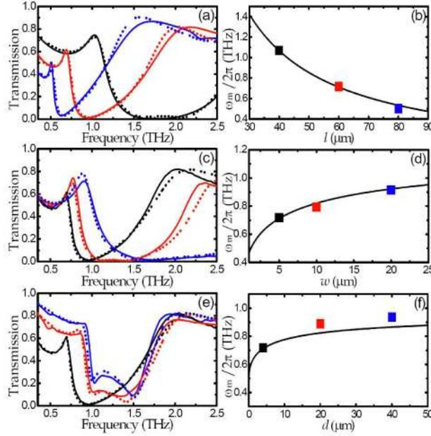
Fig. 3. Dependence of the CRP resonance on geometrical dimensions. (a), (c) and (e): measured (solid curves) and simulated (dotted curves) transmissions with (a)  $l = 40$  (black), 60 (red) and 80 (blue)  $\mu\text{m}$ . (c)  $w = 5$  (black), 10 (red) and 20 (blue)  $\mu\text{m}$ , and (e)  $d = 4$  (black), 20 (red), and 40 (blue)  $\mu\text{m}$ , respectively. (b), (d) and (f): predicted (solid curves, by the circuit model) and simulated (squares) resonance frequencies.
