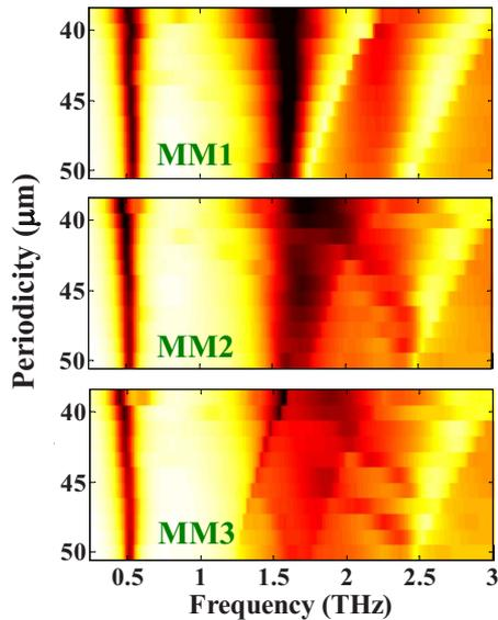
FIG. 2. (Color online) Simulated transmission of samples MM1, MM2, and MM3 as a function of the periodicity for an incident  $E$ -field perpendicularly polarized to the gap-bearing sides of the SRRs.
