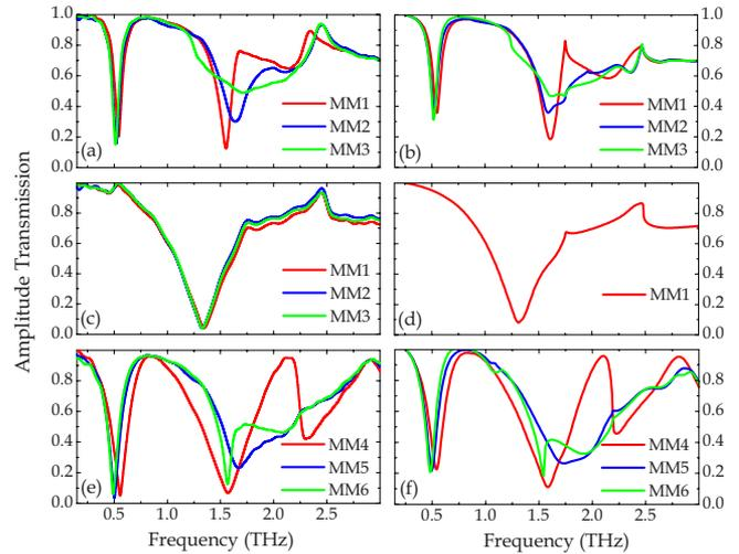
FIG. 3. (Color online) (a) Measured and (b) simulated transmission spectra of samples MM1–MM3; the incident  $E$ -field is polarized perpendicular to the gap-bearing sides of the SRRs. (c) Measured spectra of MM1–MM3 and (d) simulated spectrum of MM1 with the incident  $E$ -field polarized parallel to the gap-bearing sides. (e) Measured and (f) simulated spectra of MM4–MM6.
