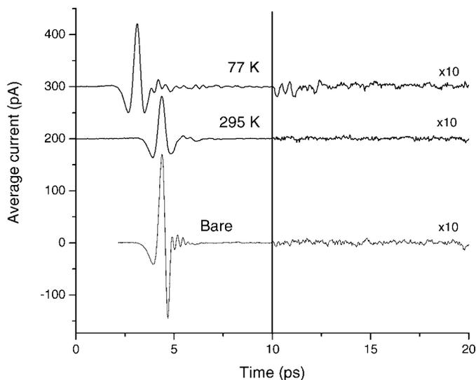
FIG. 3. THz pulses transmitted through bare Cu waveguide and the same waveguide with aspirin film at both 295 K and 77 K. Traces are multiplied by a factor of 10 after 10 ps.
