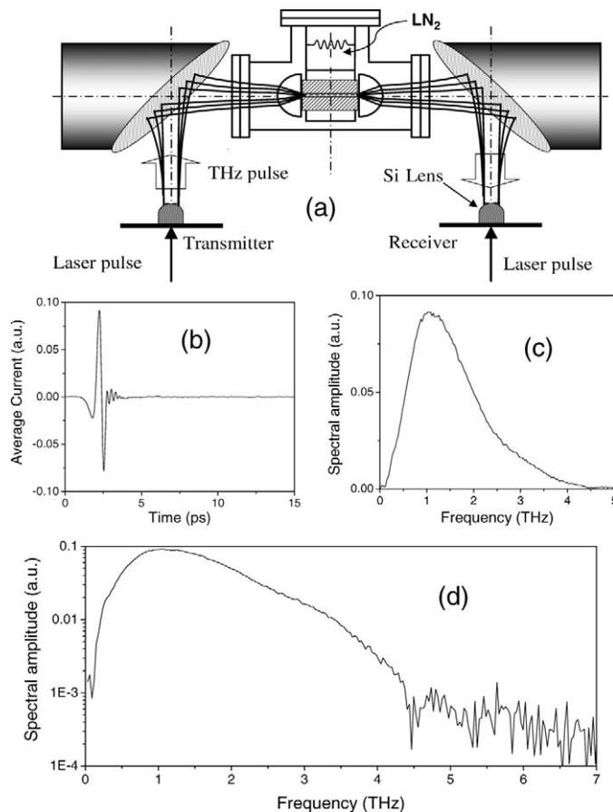
FIG. 2. (a) Waveguide THz-TDS apparatus. THz pulse transmitted through 30 mm long Cu waveguide with 50  $\mu\text{m}$  gap normalized to free-space signal in Fig. 1d (b) and corresponding amplitude spectrum normalized to free-space spectrum with both (c) linear and (d) logarithmic vertical scales.
