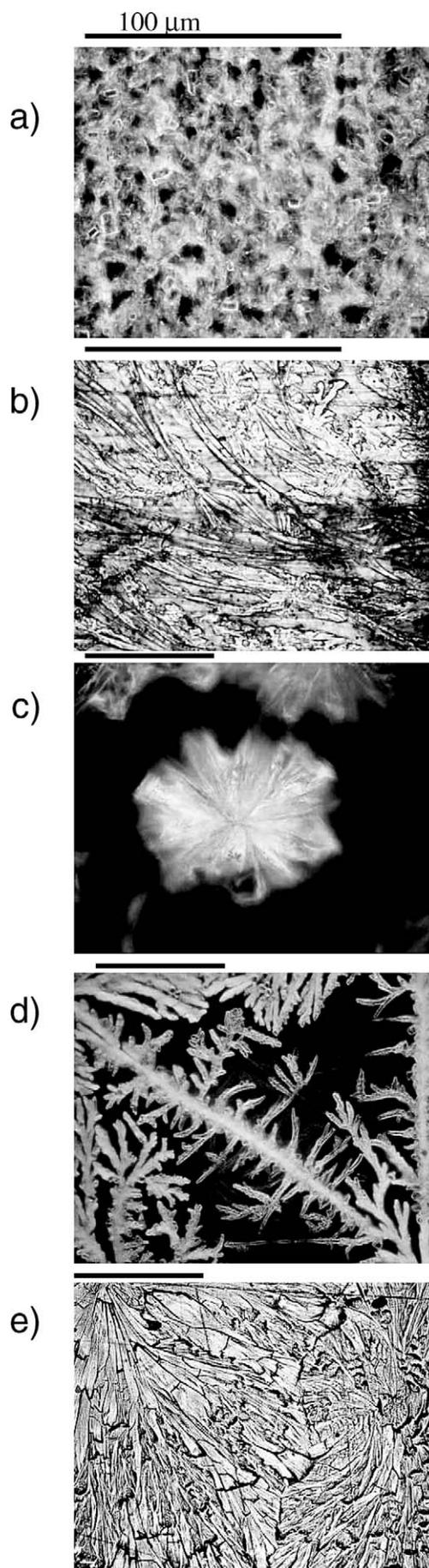
FIG. 4. Optical micrographs of measured polycrystalline films on metal waveguide plates. Horizontal lines correspond to 100  $\mu\text{m}$ . (a) Benzoic acid film on brushed Al plate. (b) Salicylic acid film on polished Cu plate. (c) 3-Hydroxybenzoic acid film on polished Al plate, image is negative for clarity. (d) 4-Hydroxybenzoic acid film on polished Al plate, image is negative for clarity. (e) Aspirin film on polished Cu plate.
