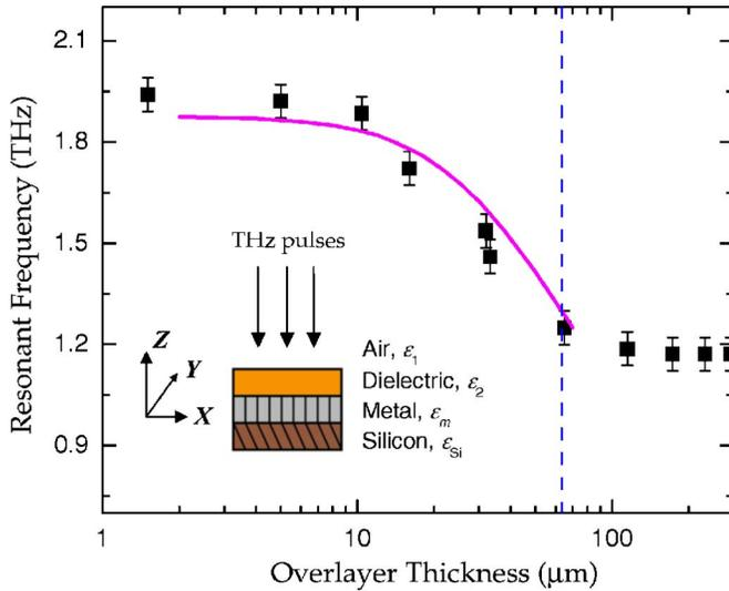
FIG. 3. (Color online) Resonant frequencies of the Al-air  $[\pm 1, 0]$  mode as a function of the thickness of the overlayer dielectric film. Experimental data: squares; numerical calculation: solid curve. Inset: schematic of the metal-dielectric interfaces of the array system.
