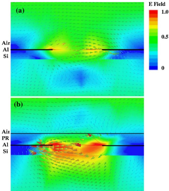
FIG. 6. (Color online) Comparison of modeled electric field by FEM at 0.5 THz, the Al-Si (AS)  $[\pm 1, 0]$  mode, without (a) and with (b) the 65  $\mu\text{m}$  thick dielectric overlayer.
