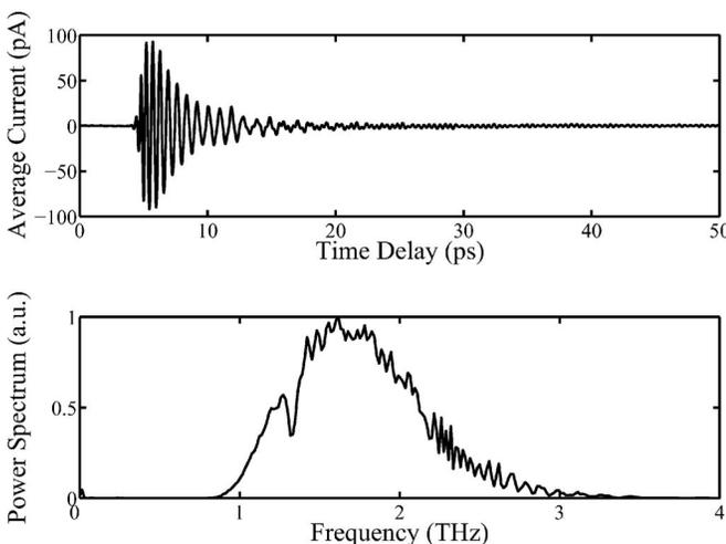
FIG. 3. Measured terahertz time-domain electric field waveform and accompanying power spectrum after propagation through a resonator structure ( $d=125$   $\mu\text{m}$  and  $w=100$   $\mu\text{m}$ ). The resonance dip at 1.331 THz is evidence of excitation of the resonator mode.
