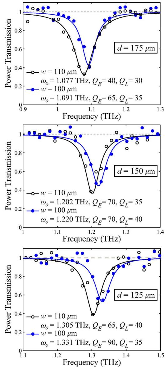
FIG. 4. (Color online) Microcavity transmission spectra for resonators with  $d=175$ , 150, and 125  $\mu\text{m}$  and average  $w=110$  and 100  $\mu\text{m}$ . Measured values  $Q_E$  are between 40 and 90 and a data extraction error of less than 10% is expected.
