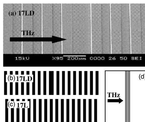
FIG. 1. (a) SEM picture of the grooved structure with center defect of chip 17LD. The period is 160  $\mu\text{m}$ , the groove width is 75  $\mu\text{m}$ , and the center groove defect width is 150  $\mu\text{m}$ . (b) Schematic of 17 period pattern with defect, chip 17LD. (c) Schematic of 17 period pattern, chip 17L. The 20  $\mu\text{m}$  deep grooves are shown in black. (d) Chip layout.
