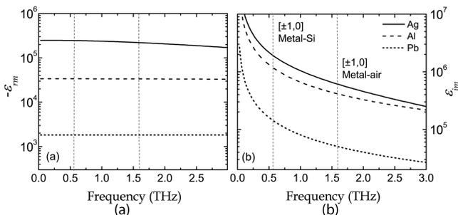
Fig. 1. Frequency-dependent Drude model dielectric constants of Ag, Al, and Pb in the THz region (Ref. 8): (a) real dielectric constant  $-\epsilon_{rm}$ ; (b) imaginary dielectric constant  $\epsilon_{im}$ . The vertical dashed lines indicate the observed  $[\pm 1, 0]$  metal-Si resonance mode at 0.55 THz and the  $[\pm 1, 0]$  metal-air mode at 1.60 THz.
