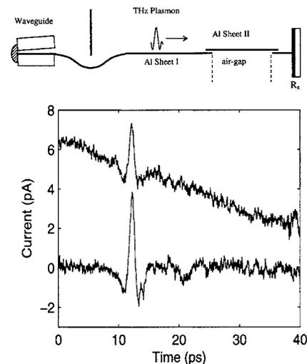
FIG. 3. Comparison of air propagated (upper pulse) and Al sheet II propagated (lower pulse) TSP. The upper figure shows the experimental setup.
