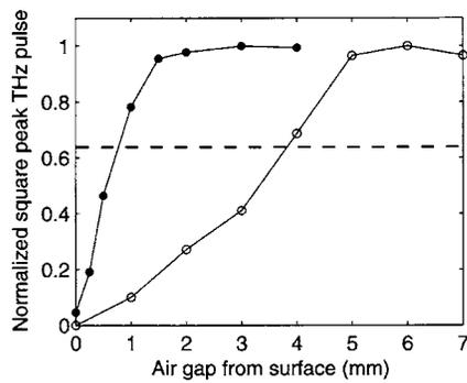
FIG. 4. Normalized measurements of the square of the peak TSP pulse amplitude vs slit opening  $Z_I$  at the center of the 6-mm-deep curve (dots), and the square of the peak TSP pulse amplitude vs slit opening  $Z_{II}$  at the center of the 15.7-cm-long Al sheet II (open circles).
